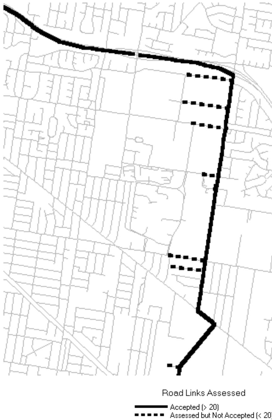
**Figure 3 Mapping GPS data to road links: accepted and not accepted points**
